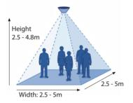
Narrower 40° lenses are available that are suitable for ceilings between 4 - 7.5m. For outdoor applications a 20° lense is also available that has a range of 7 - 12m.
