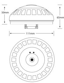
Standard Beonic Thermal Sensors have a 60° field of view, making them suitable for ceiling heights between 2.5 - 4.8m.
